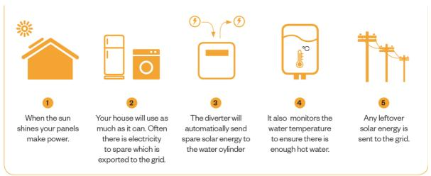
The hot water diverter is designed to re-direct solar power that would otherwise be exported to the grid into your hot water tank. This maximises the value of the power you generate through the solar system as you are using the hot water tank similar to a battery.
